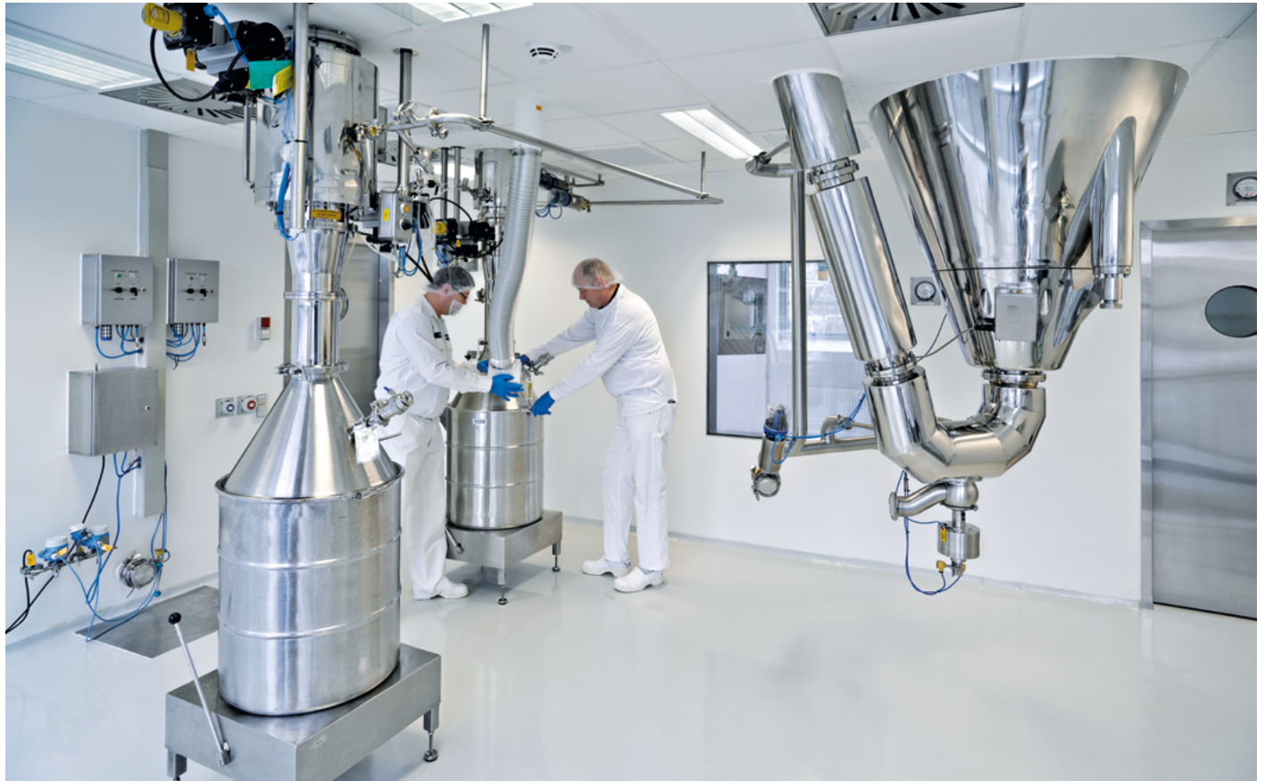
Powder collection in clean room, custom-designed PHARMA-SD® type PSD-4 at GEA Spray Drying Facility located in Soeborg, Denmark
