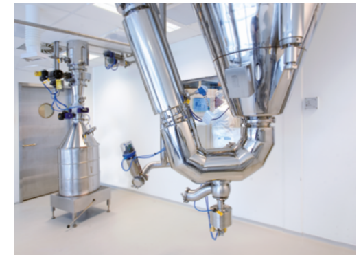
Cleaning requires a swing cone at the bottom of the drying chamber.
