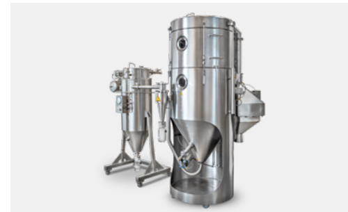
PHARMA-SD® type PSD-1 spray dryer for closed-cycle operation with solvent-based feeds. Nominal drying gas rate: 100 kg/h.
