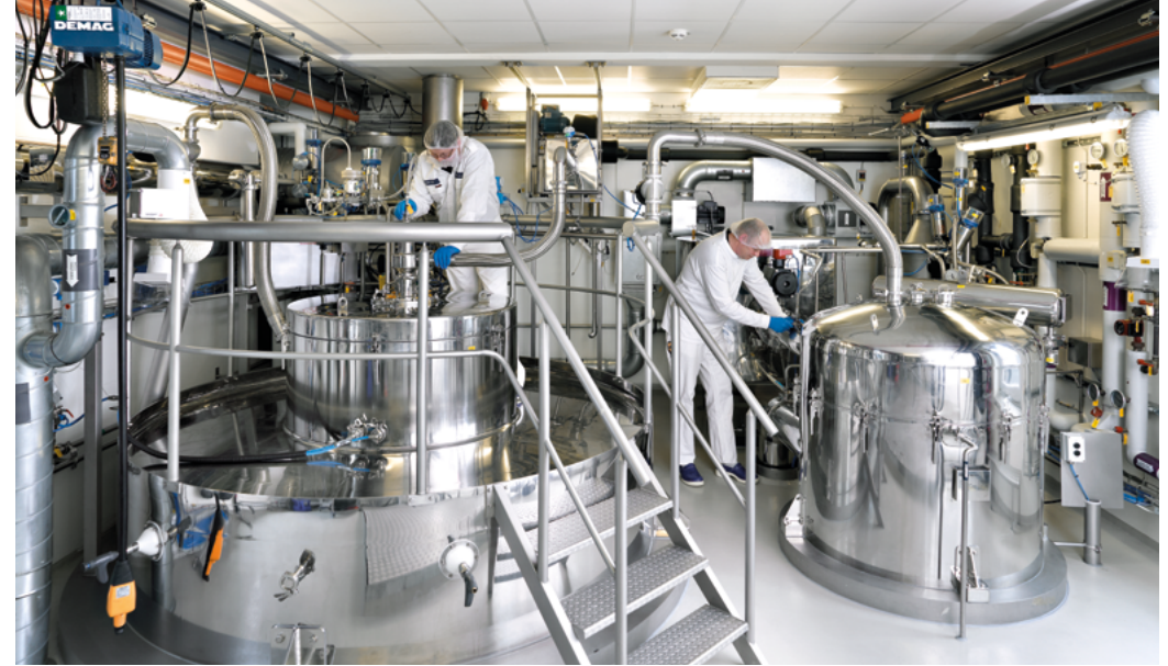
Custom-designed PHARMA-SD® type PSD-4 drying chamber roof with gas disperser and top of bag filter.
