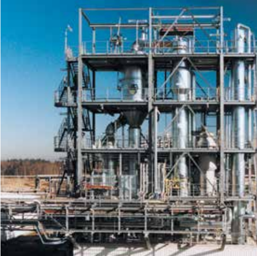
2-effect falling film, forced circulation evaporation plant in counterflow arrangement with downstream system for the purification of vapor condensate by distillation of waste water containing salts and organic compounds. Evaporation rate: 9000 kg/h concentrated to 65 % DS
