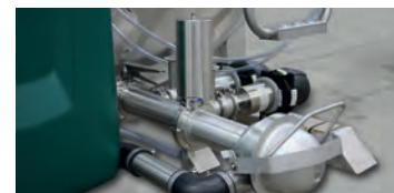
Suitable preferred connection and safe hygiene: Professional robot connection via patented 3-way valve technology separates water and milk during cleaning and milking processes.
